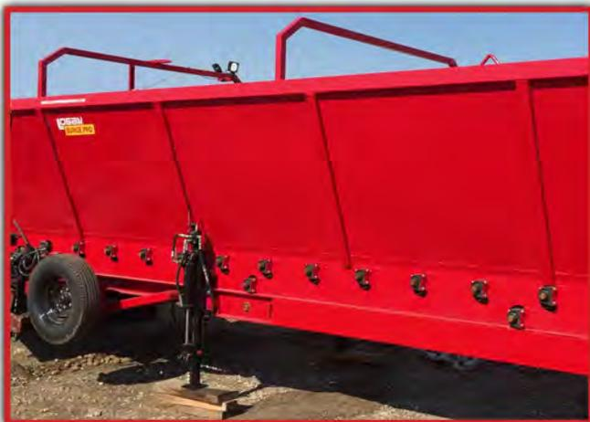
4" externally mounted discharge belt rollers provide easy access and removal. Hydraulic stabilizing jacks are also provided.
