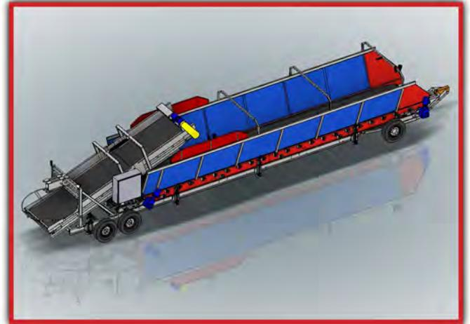
A large 54" infeed elevating conveyor, a 60" discharge belt, and a large 330 sack tank combine to give efficient production and gentle first in-first out handling. Set your output rate and the discharge belt will self adjust. The Logan Surge Pro provides a wide consistent even flow to your downstream machines improving performance!
