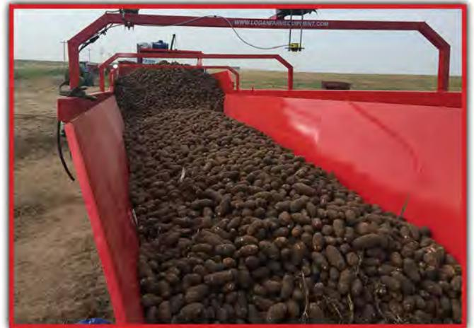
Loading the Surge Pro at the infeed end, the pile transitions lower reducing drop and rolling at discharge.
