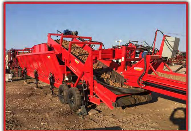
54" infeed elevating conveyor, with dual stinger hanger.
