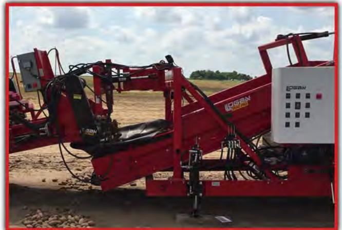
Main tandem axles closest to the intake and a single axle closest to the discharge make up the Surge Pro's chassis. Value added options include torsion axles with removable hitch, hydraulic brakes on the main axles, hydraulic lift lower, hydraulic steering, and wheel drive for the single axles.
